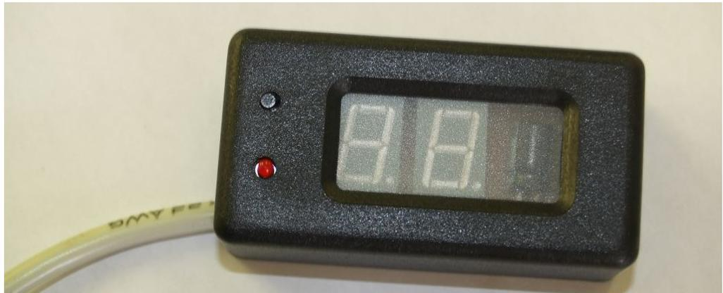
Adjusting the EFIE is a very simple process; you don't need any voltmeter or any other tool to adjust. You change the setting by pressing the button and changing the numbers.
